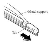
3. Remove the metal stiffener from each blade rubber and install them in the new blade.
